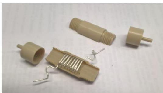
Figure 2. Sample holder for HP-<sup>129</sup>Xe-NMR measurements on porous thin films.
